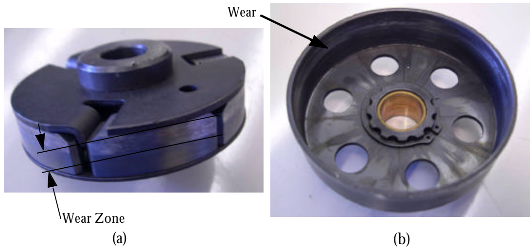
Figure 6.5 The (a) shoe and (b) drum wear of the Comet clutch. Only half of the shoe engages with the drum because the spring wraps around the shoe a little off center.
