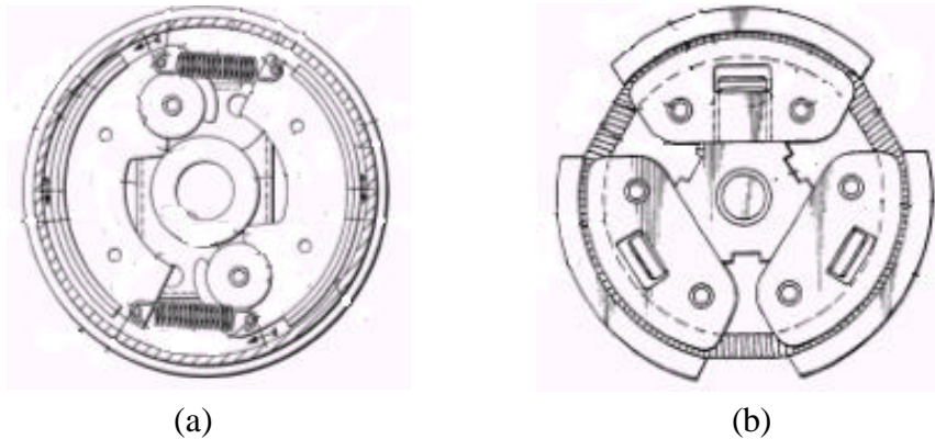
Figure 2.4 (a) St. John's [10] patented connected shoe clutch. (b) Nagashima's [11] patented floating shoe clutch.
