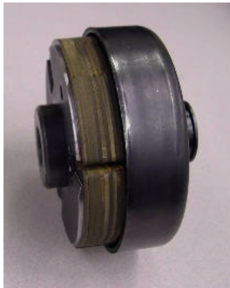
Figure 6.6 MFOA clutch assembled into a Comet drum. The clutch consist of 10 layers of spring steel: each 0.062" thick.
